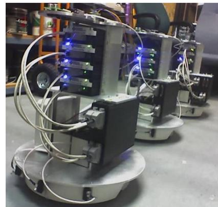
single target acquisition robot used a video sensor. All robots had IR rangefinders for collision avoidance and used Cricket sensors and odometry for positioning.
